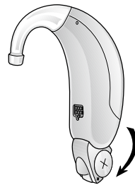
open battery door completely
