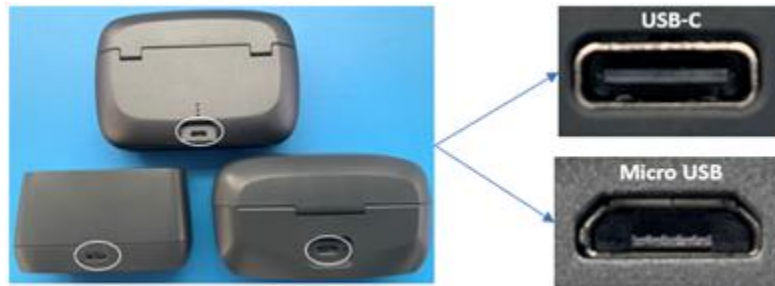
FIGURE: The above photo illustrates the chargers showing the different connectors where there can be discoloration or damage due to overheating
